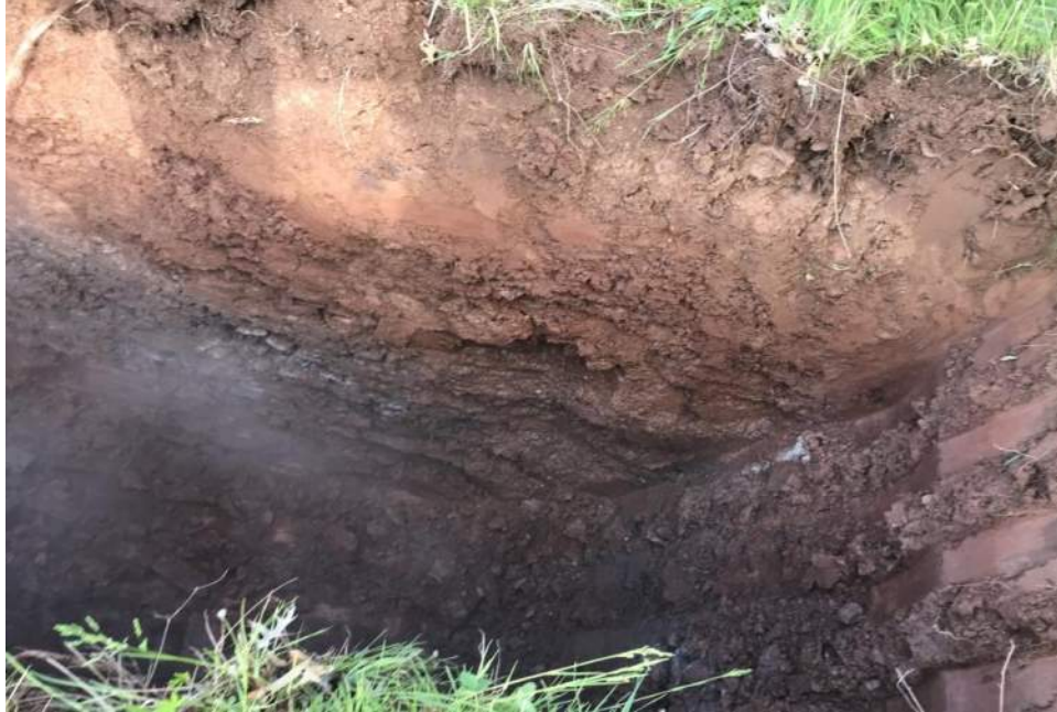
Photo 3: TP-102 Profile pit
