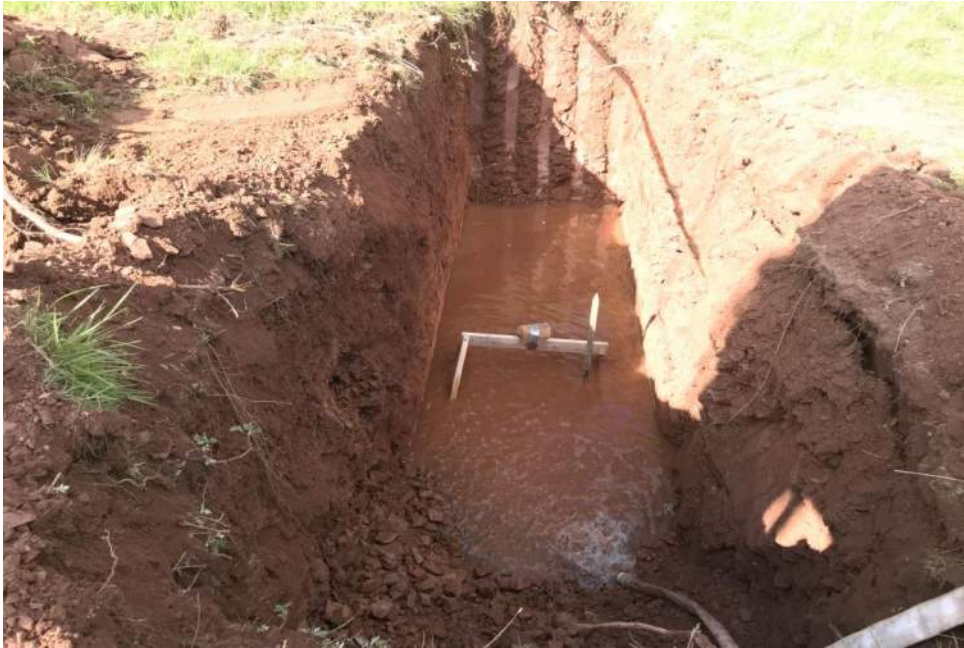
Photo 12: TP-108 Basin Flood Test set up
