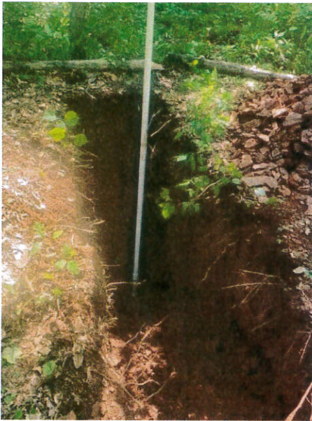
Typical Constant Head Well Permeameter Test
