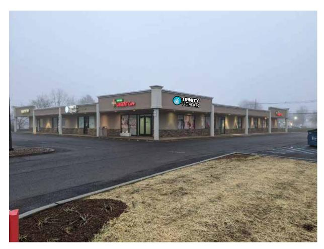
PROPOSED SIGN ARE CHANNEL LETTERS WITH ALUMINUM BODIES AND ACRYLIC FACES MOUNTED TO A BLACK ALUMINUM BACKER, FRONT LIT, USING LED LIGHTING MOUNTED TO A RACEWAY.
