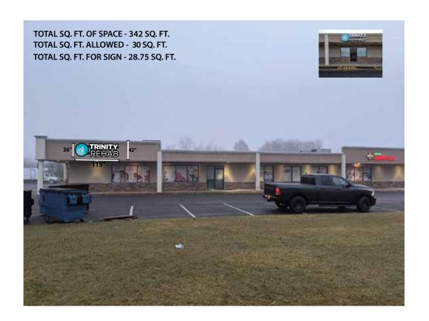
PROPOSED SIGN ARE CHANNEL LETTERS WITH ALUMINUM BODIES AND ACRYLIC FACES MOUNTED TO A BLACK ALUMINUM BACKER, FRONT LIT, USING LED LIGHTING MOUNTED TO A RACEWAY.
