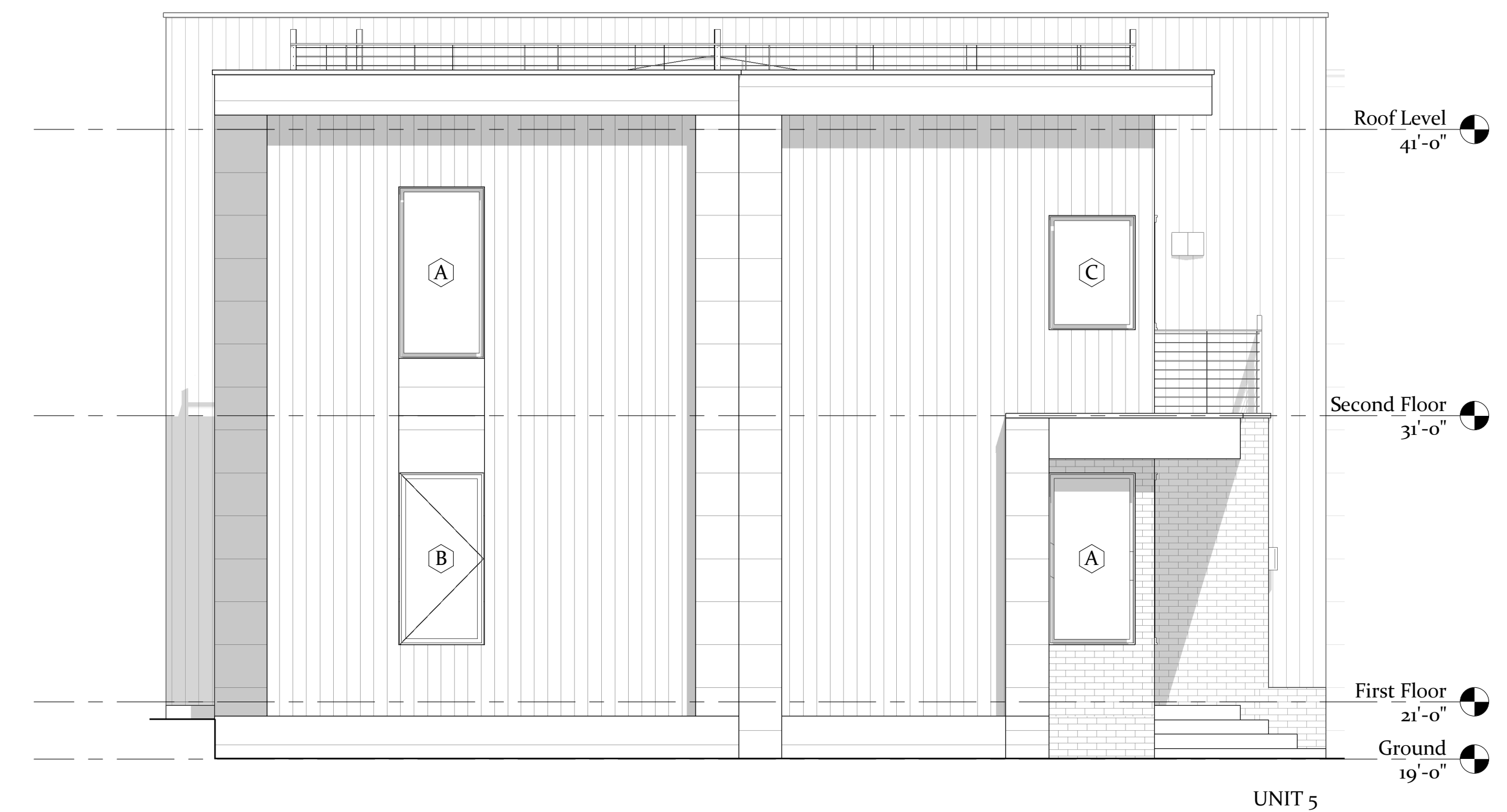
① Left Side Elevation - Units 5-6 1/4" = 1'-0"
