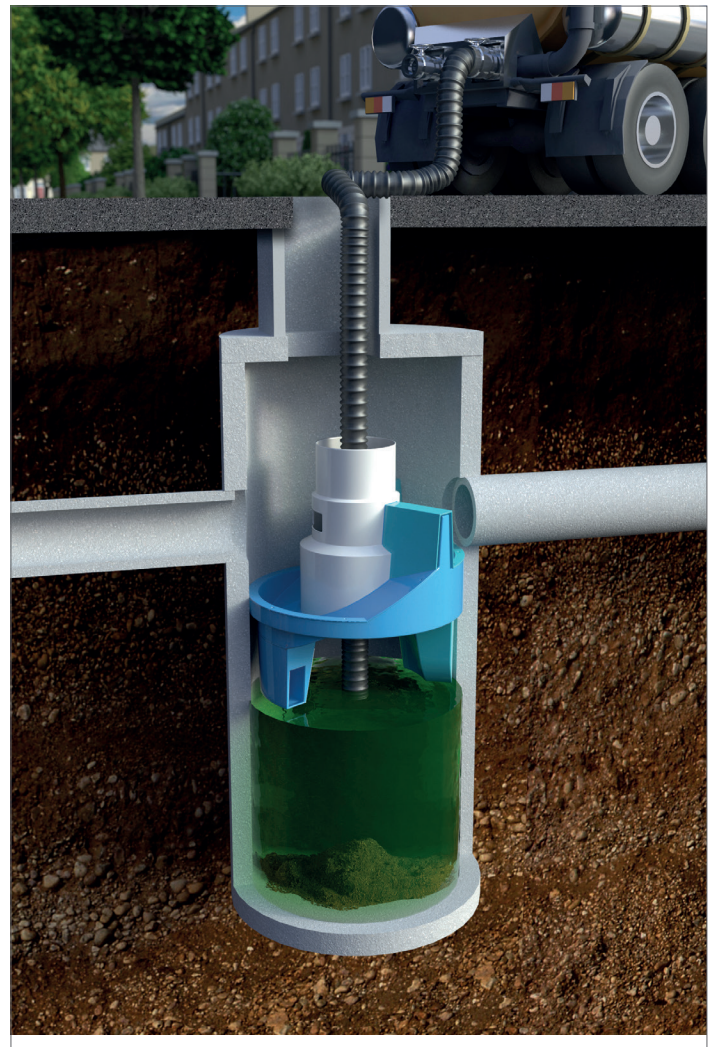
Fig.4 Floatables are removed with a vactor hose
