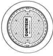
FRAME AND COVER (30" ROUND) (NOT TO SCALE)
